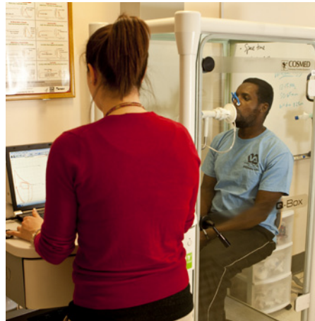
The WRIISC has many state-of-the-art assessments for Veterans with airborne hazard exposures. One of these methods is complete pulmonary function testing (PFT) which includes assessment of spirometry, lung volume, and lung diffusing capacity.
