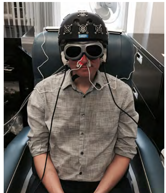
A staffer in Dr. Margaret Naeser’s lab demonstrates the equipment built especially for the research: an LED helmet (Photomedex), intranasal diodes (Vielight), and LED cluster heads placed on the ears (MedX Health). Goggles are worn to block out the red light. The near-infrared light is beyond the visible spectrum and cannot be seen. (Photo courtesy of Naeser lab)
