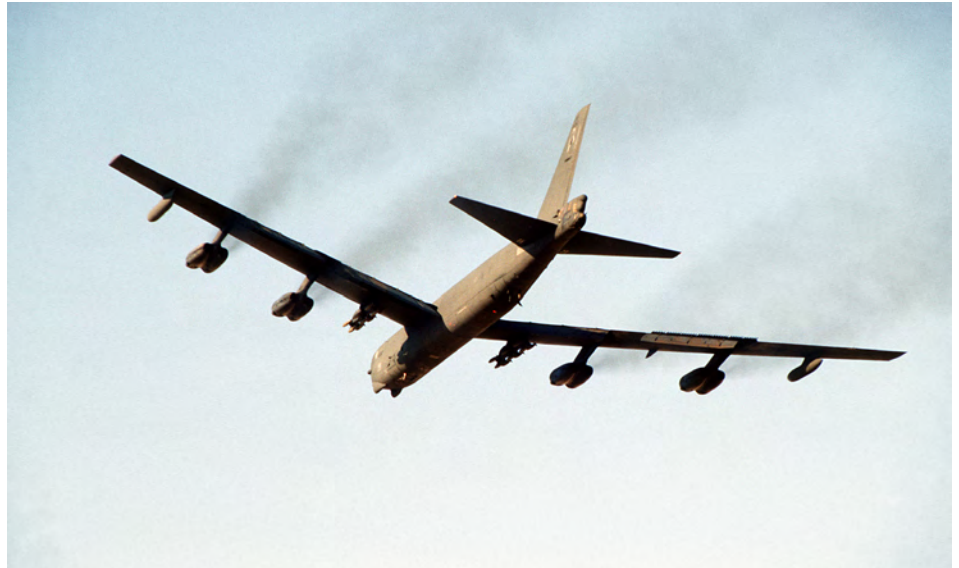
A U.S. Air Force B-52G Stratofortress aircraft takes off on a mission in support of Operation Desert Storm. The aircraft is armed with bombs on the wing pylons.
